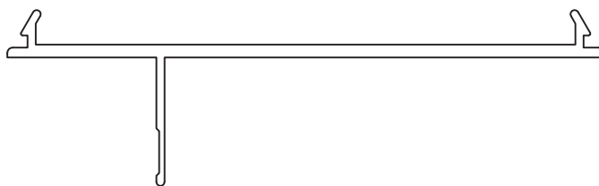
700-251 Infill - Reveal Adaptor 100mm I_{xx} = 2.66 \times 10^3 \text{ mm}^4
