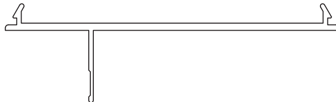
700-251 Infill - Reveal Adaptor 100mm I_{xx} = 2.66 \times 10^3 \text{ mm}^4
